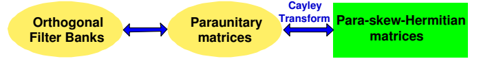
Fig. 1. One-to-one mapping between paraunitary matrices and para-skew-Hermitian matrices via the Cayley transform.
