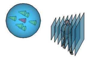
Fig. 2. The spatial extent of a NOV (sphere) with one pair of image and depth map, along with seven views (cones). The central dark cone designates the reference view. The planes represent iso-depth surfaces (3D model courtesy of Google).
