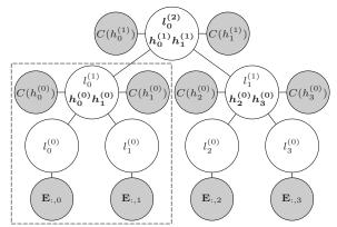
Fig. 5. Dependency graph of a three-level L transform. The coefficients in bold are those included in the wavelet vector d. Gray nodes represent the MSE and rate terms of the RD optimization. The dashed box highlights the two-level L transform associated with (22).
