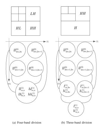
Fig. 7. Two divisions of the frequency plane and the associated graphs of dependencies between the coefficients of the S transform.
