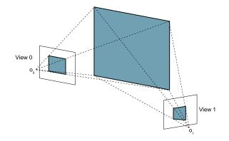
(a) A reference view s = 0 along with an arbitrary view s = 1 and an iso-depth plane.
