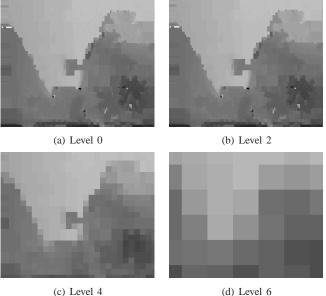
Fig. 9. Disparity map of the Teddy set at four resolution levels, showing the resolution scalability of the wavelet-based representation.
