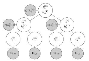
Fig. 6. Dependency graph of a three-level S transform. The coefficients in bold are those included in the wavelet vector d. Gray nodes represent the MSE and rate terms of the RD optimization.
