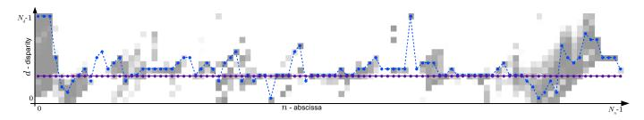
Fig. 4. An error matrix **E** from the Tsukuba image set [19] with two optimal paths overlaid,  $\lambda = 0$  (dashed) and  $\lambda = \infty$  (solid). Lighter shades of gray indicate larger squared intensity differences.
